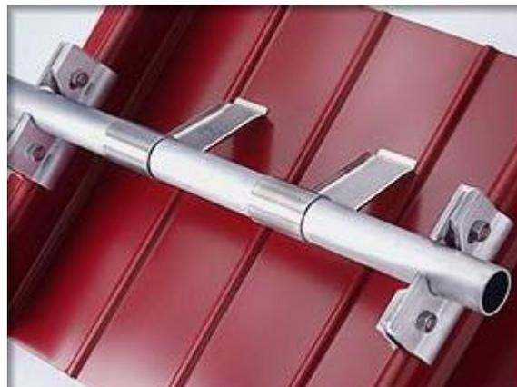
Hold the ice stopper onto the pipe as shown on the right - the open part facing toward the top of the roof -
